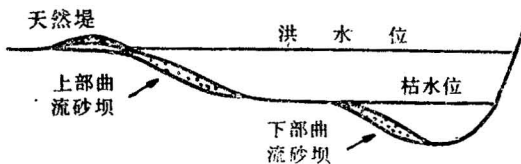
图1 阶梯状曲流砂坝河流横切面示意图 Fig. 1 Cross section of meandering stream with stepped profile point bar surfaces
