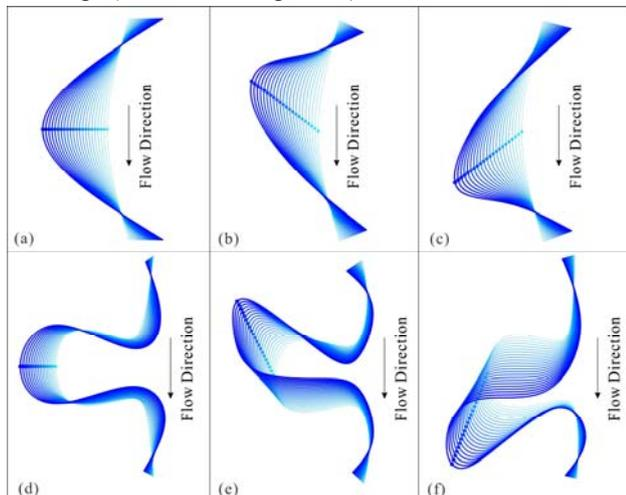
Fig. 1. Geomorphology planform migration processes of meandering channel under ideal conditions.
