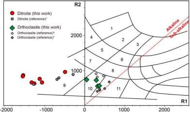
Fig. 1. Chemical classification of the Jebel Dumbier alkaline rocks after de la Roche's (1986). R1=4Si-11(Na+K)-2(Fe+Ti), R2=6Ca+2Mg+Al. 1. melteigite; 2.theralite; 3. alkali gabbro; 4. ijolite; 5. essexitic gabbro; 6. syenogabbro; 7. essexite; 8. nepheline syenodiorite; 9. nepheline syenite; 10. nepheline-bearing syenite; 11. syenite.
