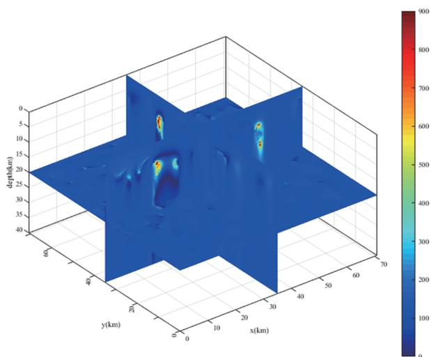
Fig. 4. Cross section intersected from the 3D imaging in Fig. 5. The cross sections of the gravity imaging results by continued fraction downward continuation from the airborne anomaly in Fig. 5 at  $x = 35 \text{ km}$ ,  $y = 35 \text{ km}$ , and  $z = 20 \text{ km}$ .
