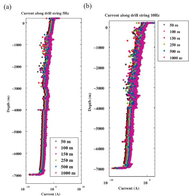
Fig. 2 Comparison of current distribution along the drill string in cased well at frequencies.
