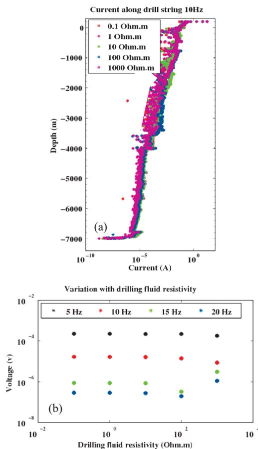
Fig. 3. Results obtained by varying the drilling fluid resistivity value.
