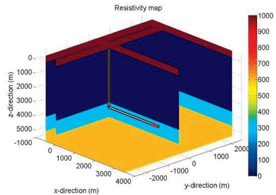
Fig. 1. 3D geological model showing the horizontal well and subsurface formation distribution. The insulating gap position on the drill string was indicated by a red mark close to the drill bit.
