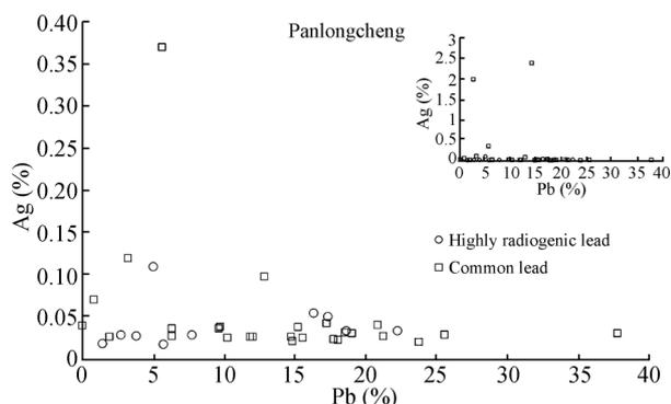
Fig. 10. A plot of %Ag vs %Pb in the bronzes from Panlongcheng (Chen et al., 2001; Sun et al., 2001; Peng et al., 2001), classified as either highly radiogenic or common lead using cut-off of  $^{206}\text{Pb}/^{204}\text{Pb}=19$ .
