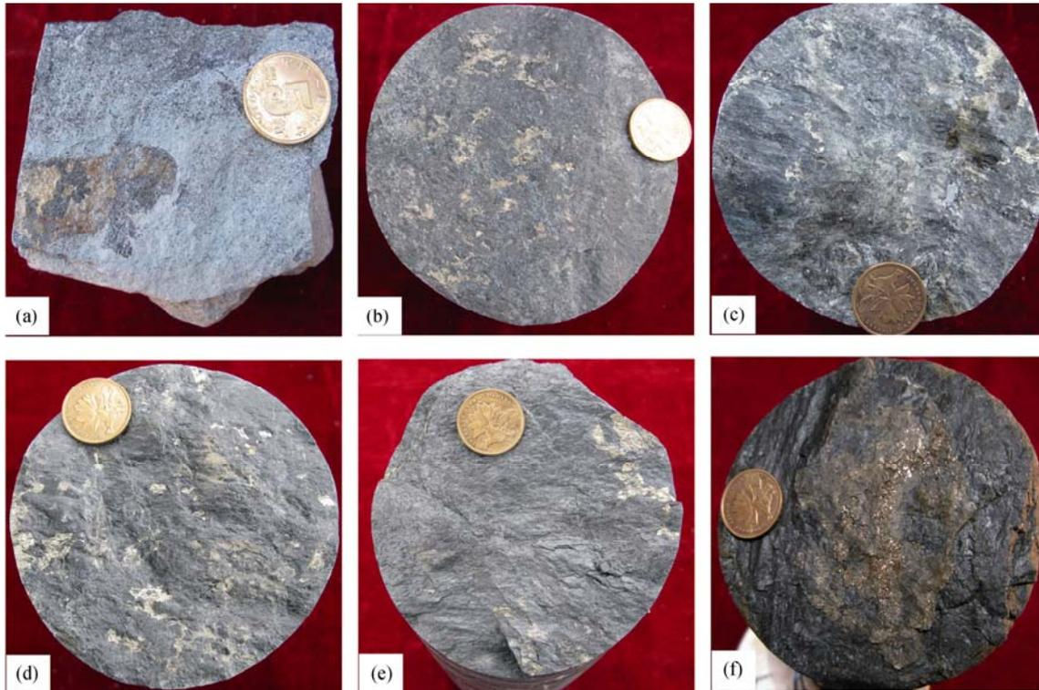
Fig. 5. Pyrite on fissured surfaces of Mk-2 well drilled cores of the Mohe Basin, northeast China. (a), Film-shape pyrite on the crevice surface (36.5–38.65 m); (b), film-shape pyrite on the bedding surfaces (53.4–56.05 m); (c), film-shape pyrite on the fracture surface (62.6–67.53 m); (d), film-shape pyrite on the bedding surface (149.85–150.05 m); (e), film-shape pyrite on the bedding surface (151.2–151.4 m); (f), grain-shape pyrite on the fracture surface (229.5–241.45 m).
