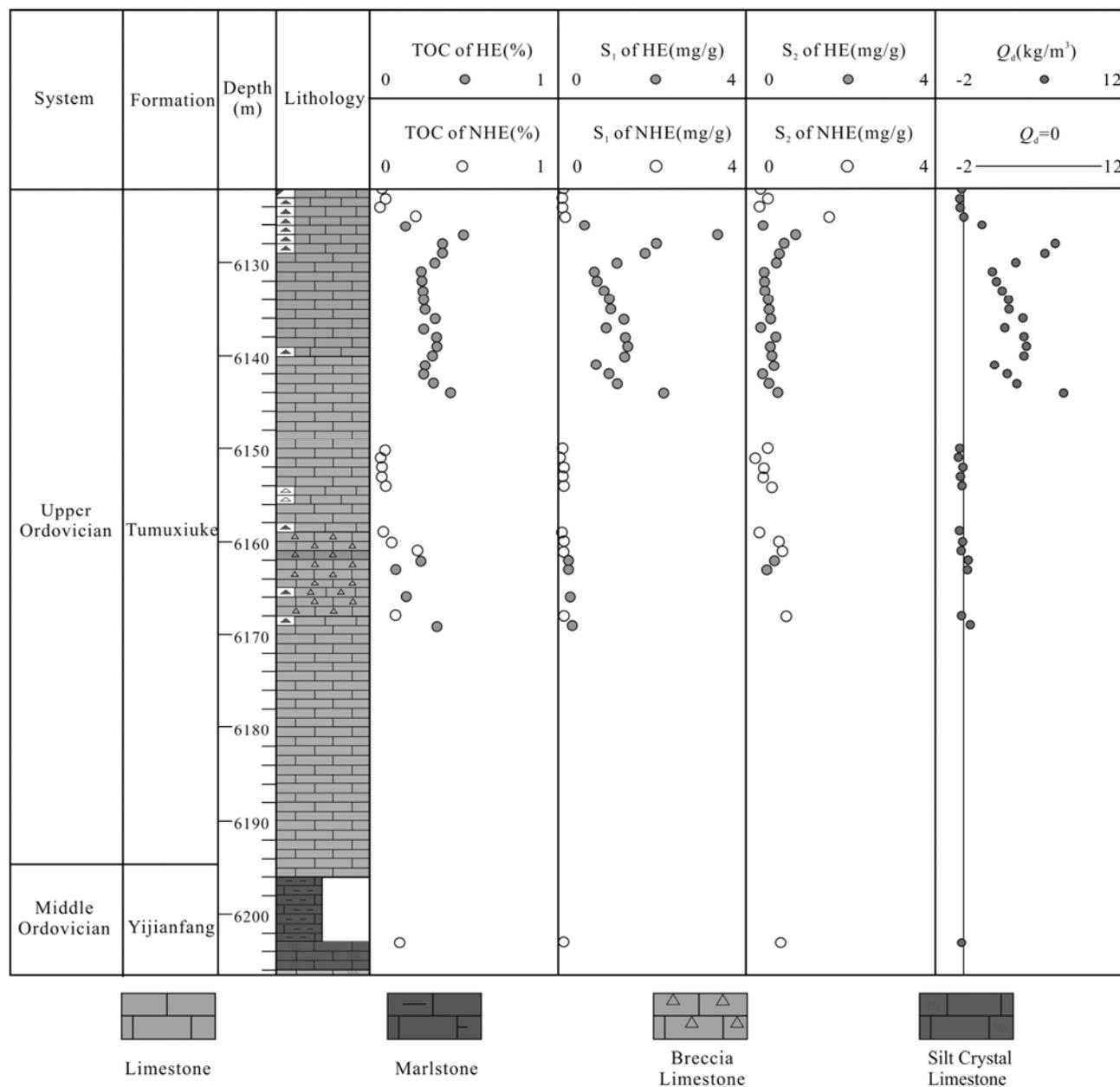
Fig. 6. Identification results and characteristics of the present-day low-TOC carbonate source rock in the Middle–Upper Ordovician in the LN46 well (location is shown in Fig. 1a). In the figure, HE means carbonates have hydrocarbon expulsion during their history and NHE means carbonates have no hydrocarbon expulsion.
