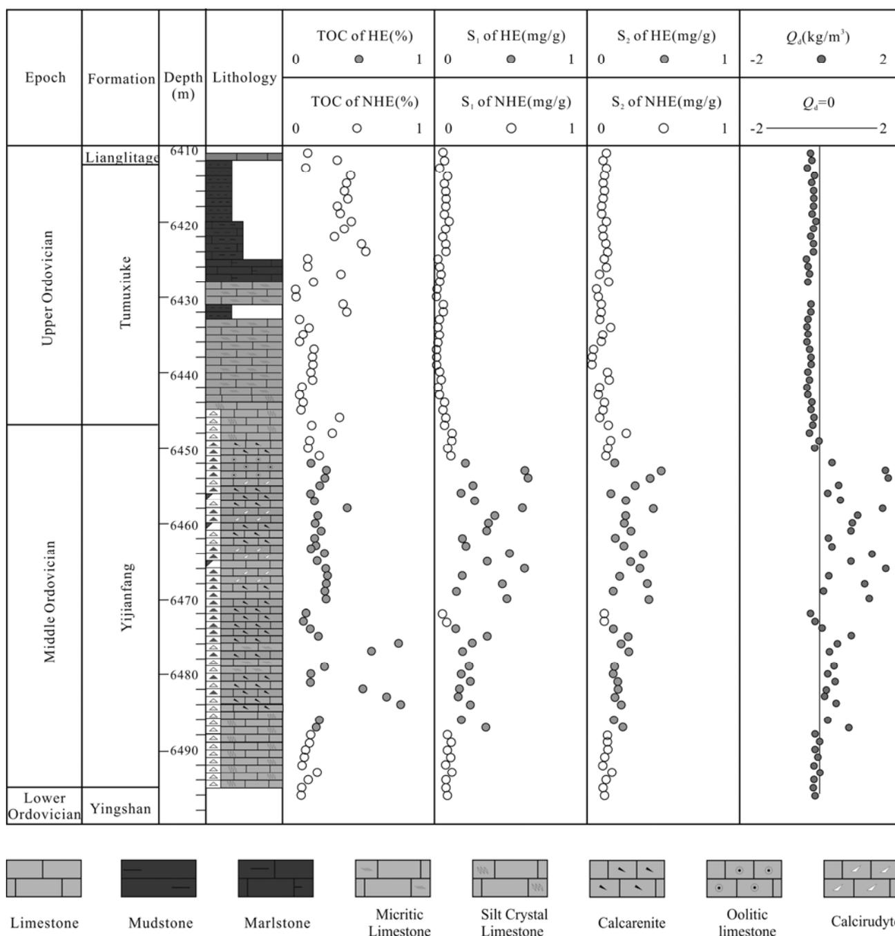
Fig. 5. Identification results and characteristics of the present-day low-TOC carbonate source rock in the Middle–Upper Ordovician in the YW2 well (location is shown in Fig. 1a). In the figure, HE means carbonates have hydrocarbon expulsion during their history and NHE means carbonates have no hydrocarbon expulsion.
