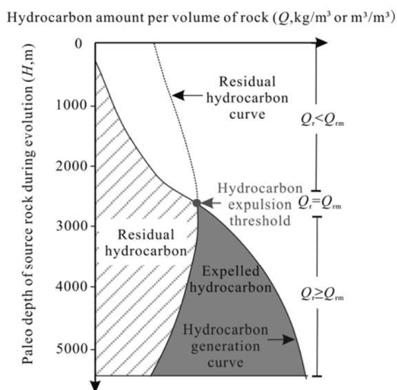
Fig. 2. Model showing mass balance of hydrocarbon generation, retention and expulsion of source rocks (modified from Pang et al., 2005).
