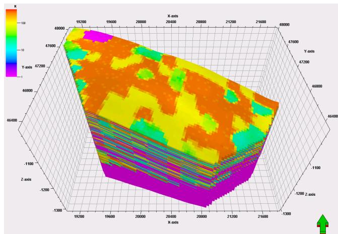
Fig.1 the permeability model of the test site
