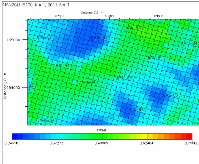
Fig. 7 the remaining oil of local-worse and channel-edge type
