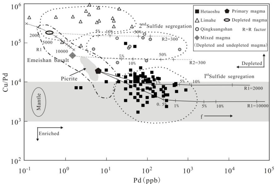
Fig. 1 Pd vs Cu/Pd diagram of typical Ni-Cu-PGE magmatic sulfide deposits in ELIP. Primitive mantle values after Sun and McDonough, 1989; Emeishan picrites and basalts from Zhong et al., 2006; Limahé from Tao et al., 2008; Qingkuangshan from Zhu et al., 2012; Partial Hetaoshu sulfide ore from 601 Geological Brigade of Sichuan company of Metallurgical Geology & Exploration, 1974; f, content of segregated sulfide.
