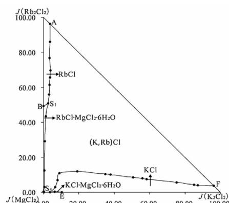
Fig. 3. Metastable phase diagram of quaternary system  $K^+, Rb^+, Mg^{2+} // Cl^- - H_2O$  at 323 K.
