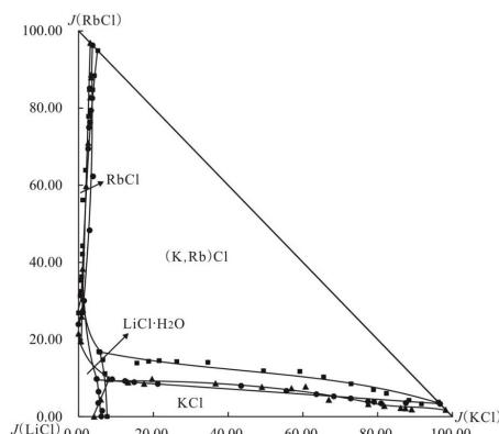
Fig. 2. Metastable phase diagram of quaternary system  $Li^+, K^+, Rb^+ // Cl^- - H_2O$  at (298, 323 and 348) K ( $\blacktriangle$  298 K,  $\bullet$  323 K,  $\blacksquare$  348 K).
