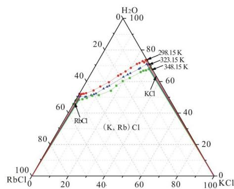
Fig. 1. Metastable phase diagram of ternary system  $KCl + RbCl + H_2O$  at (298, 323 and 348) K.
