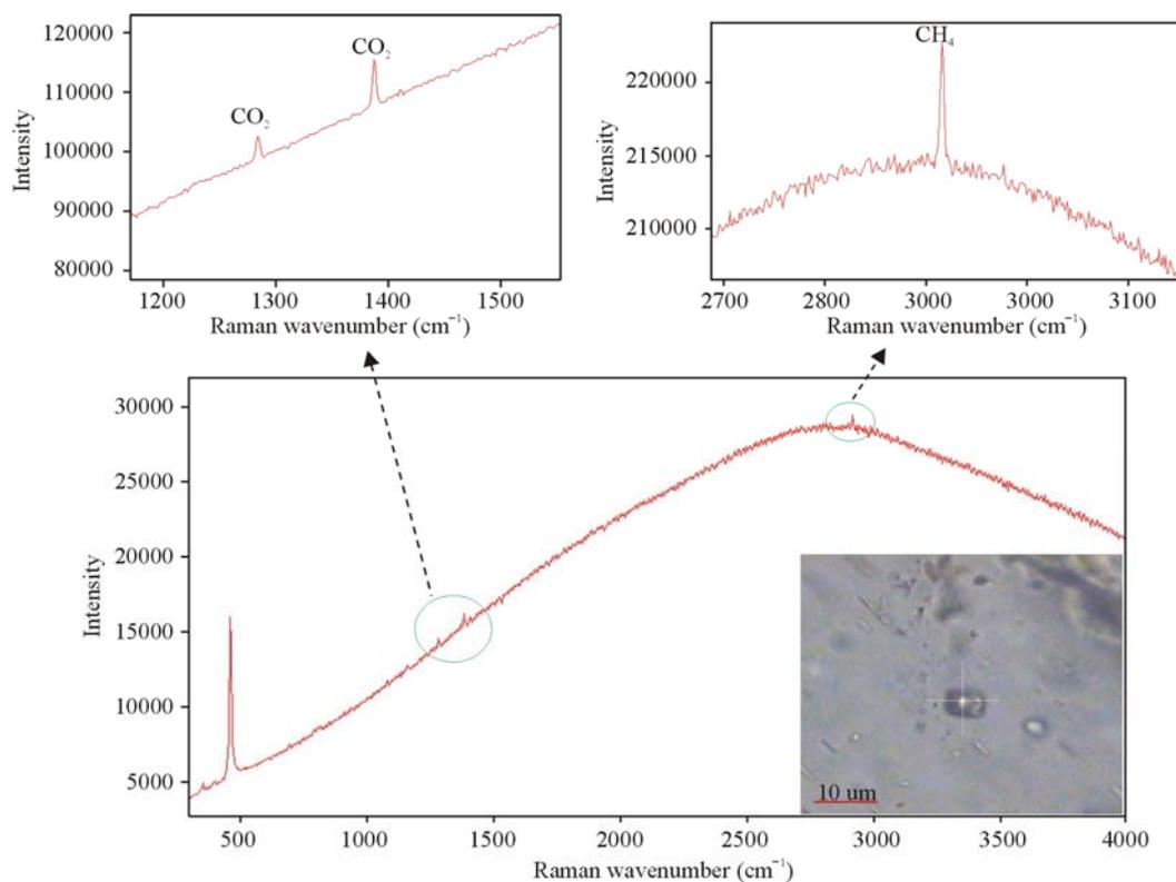
Fig. 3. Laser Raman spectra showing CH<sub>4</sub> and CO<sub>2</sub> in gaseous inclusions in A3–15.
