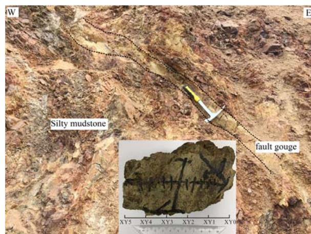
Fig. 1. Occurrence of the fault gouge (dotted line) showing injection structure. the relative samples were labeled as XY0, XY1, XY2, XY3, XY4, XY5 from one side of the fault gouge to another
