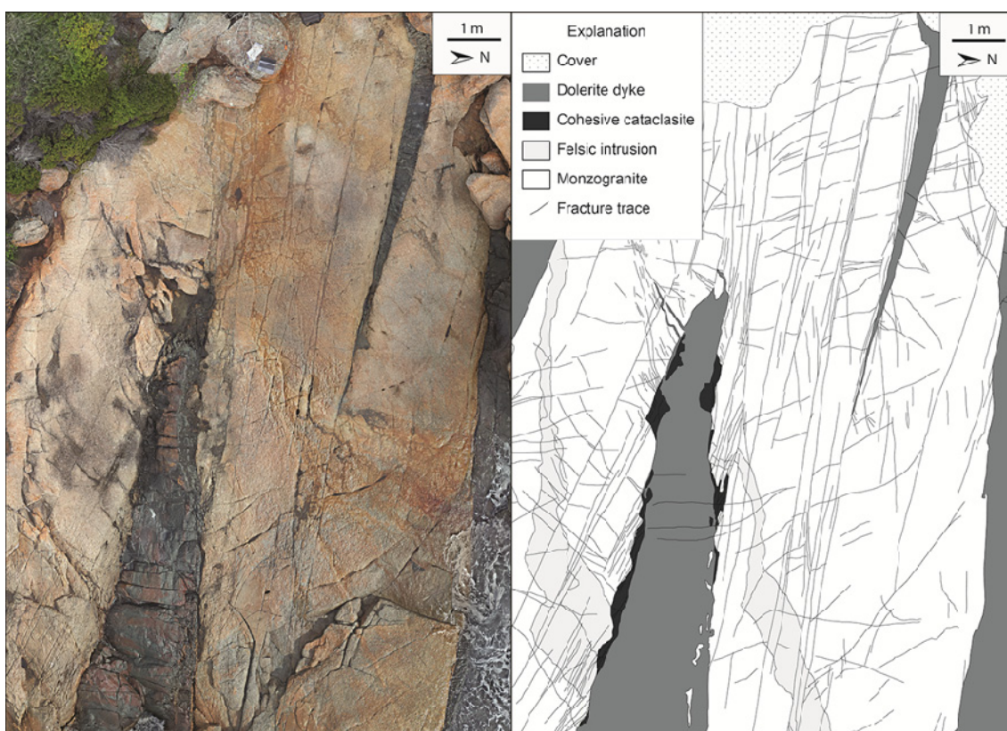
Fig. 1. High resolution UAV photogrammetry orthoimage of dyke tips emplaced in granitic host rock (left). Geologic map of same outcrop showing relations of dykes to faults and fractures (right).
