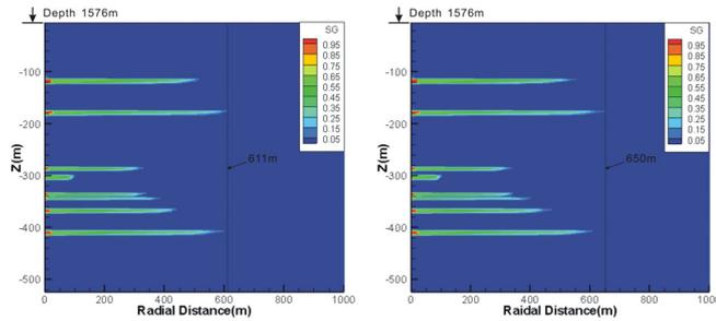
Fig. 5 Gas saturation after 20 years' CO<sub>2</sub> injection (a) Not considering Mechanical effect (b) Considering Mechanical effect
