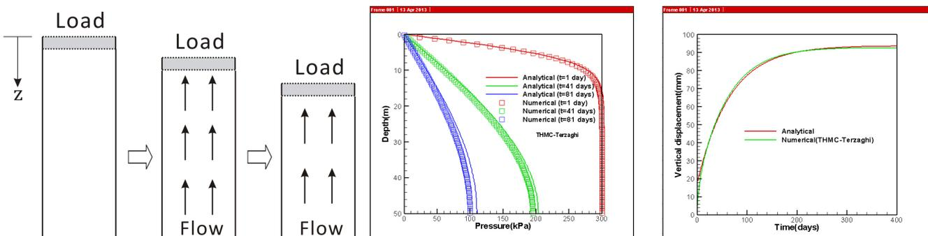
Fig. 2 Conceptual model and results comparison for one-dimension consolidation (a) Pressure (b) Displacement
