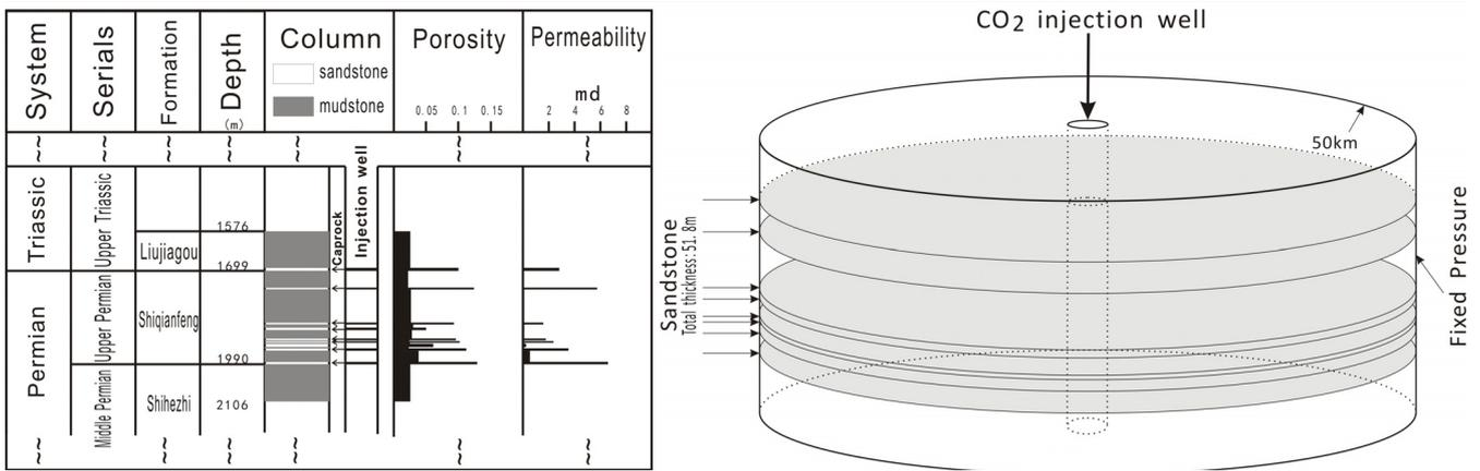
Fig. 3 Characteristic of Shiqianfeng–Liujigou reservoir-caprock formations and conceptual model for THMC processes (a) Shiqianfeng–Liujigou reservoir-caprock formations (b) Conceptual model for THMC processes
