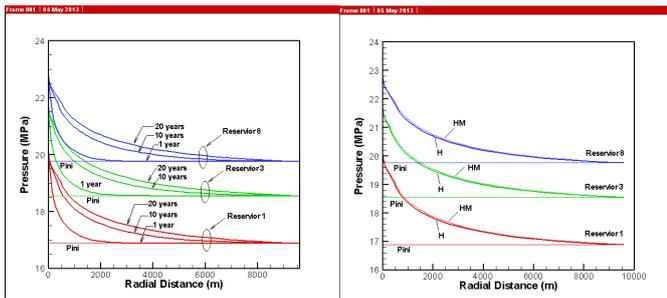
Fig. 4 Change in pressure induced by CO<sub>2</sub> injection
