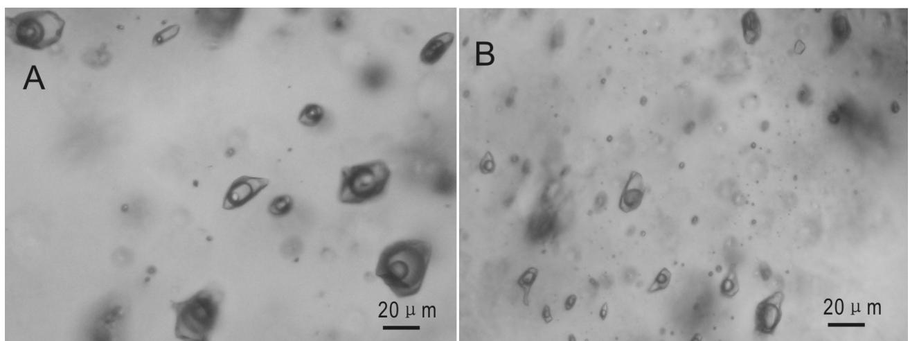
Figure 3 Fluid inclusions in quartz veins of gold deposits in the Dongtongyu gold deposit
