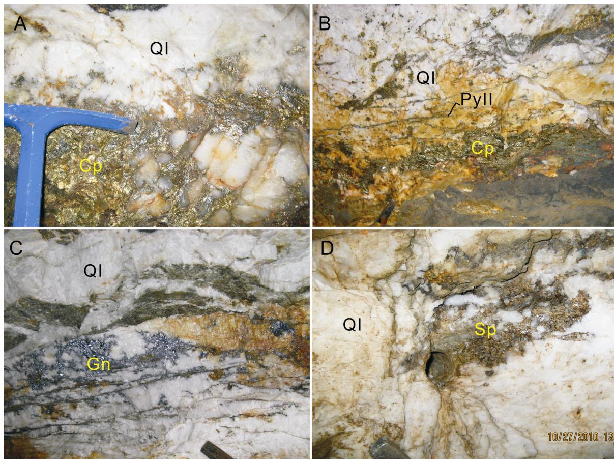
Fig.2 Characteristics of gold-bearing quartz veins in the Dongtongyu gold deposit
