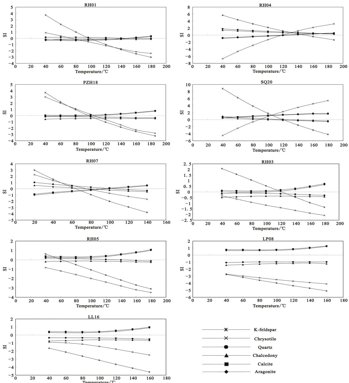
Fig. 3 Log (Q/K)-T diagrams for geothermal water samples
