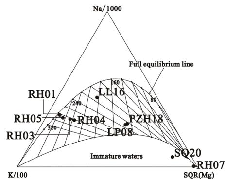
Fig. 2 Triangular Na-K-Mg diagram for geothermal water samples from Tengchong
