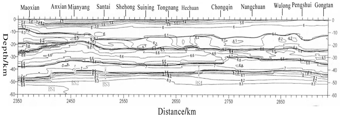
Fig.6. The velocity profile of Sichuan Maowen - Chongqing Gongtan
