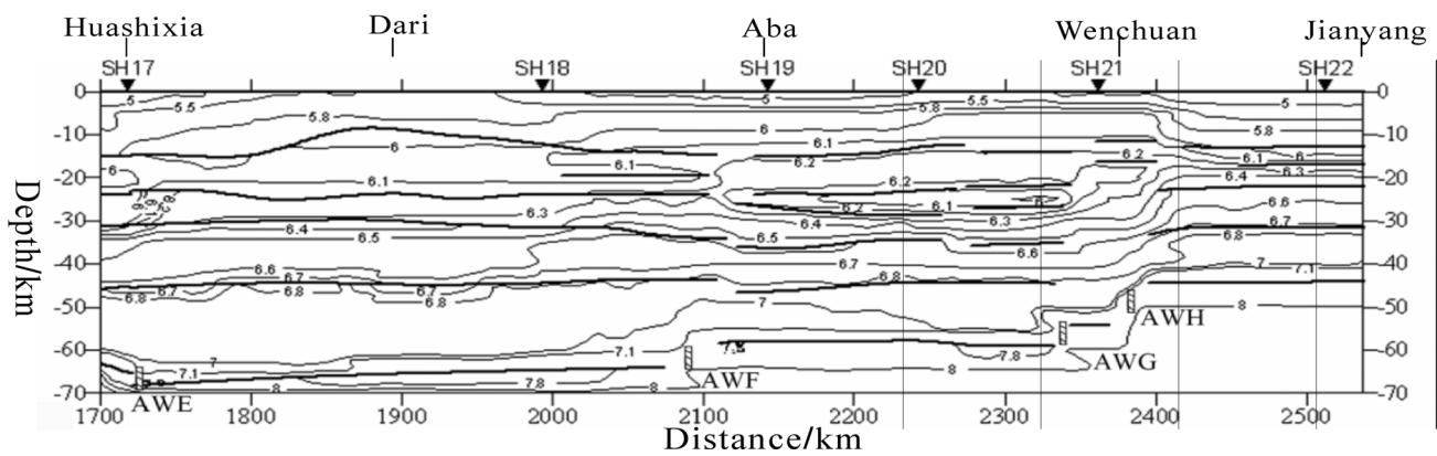
Fig.7. The velocity profile of Qinghai, Huashixia-Sichuan Jianyang
