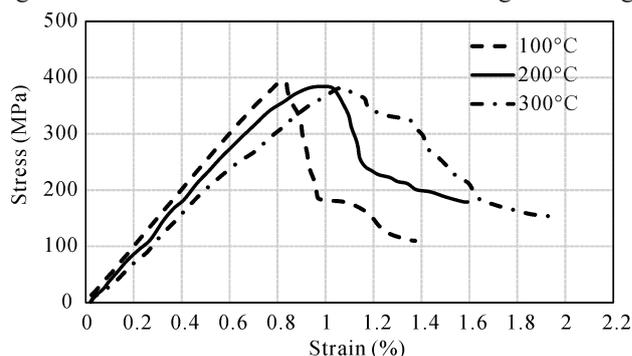
Fig. 2. Stress–strain curves under different temperatures and confining pressures.
