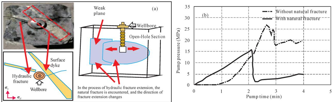
Fig. 5. Fracture creation under large horizontal stress difference (a), and small horizontal stress difference (b).
