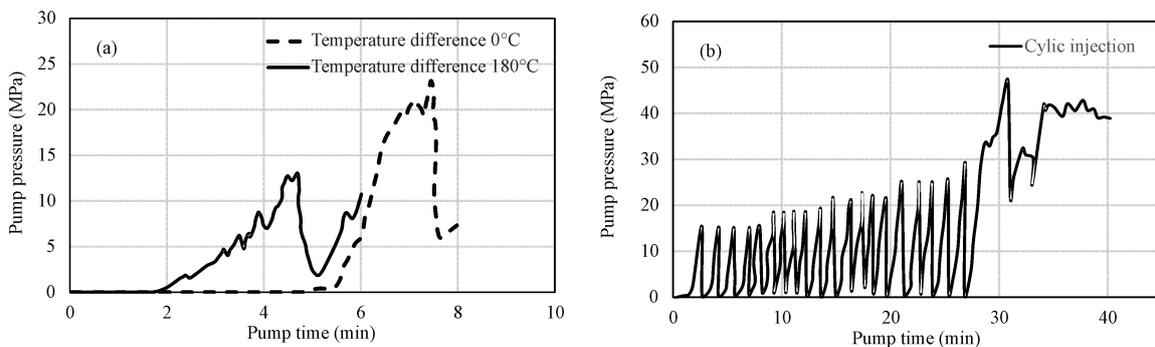
Fig. 4. Effect of temperature difference on fracture initiation pressure (a), and alternative cyclic injection (b) at low displacement on fracture initiation pressure.
