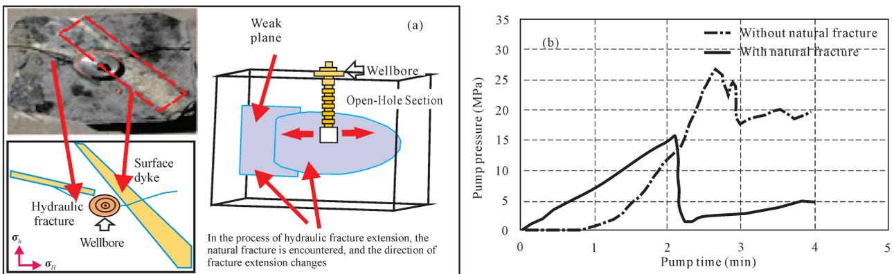
Fig. 3. Hydraulic fracture extension physical picture (a) and injection curve (b).
