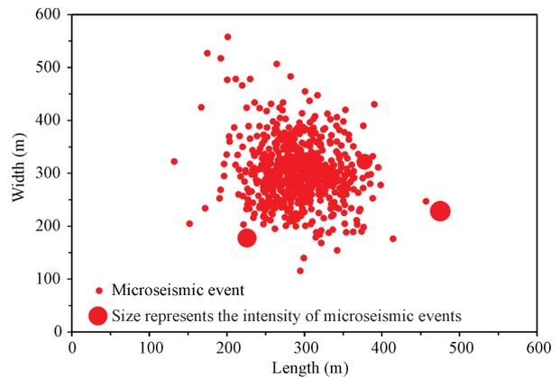
Fig. 6. Micro-seismic events in well X1 during fracturing treatment.
