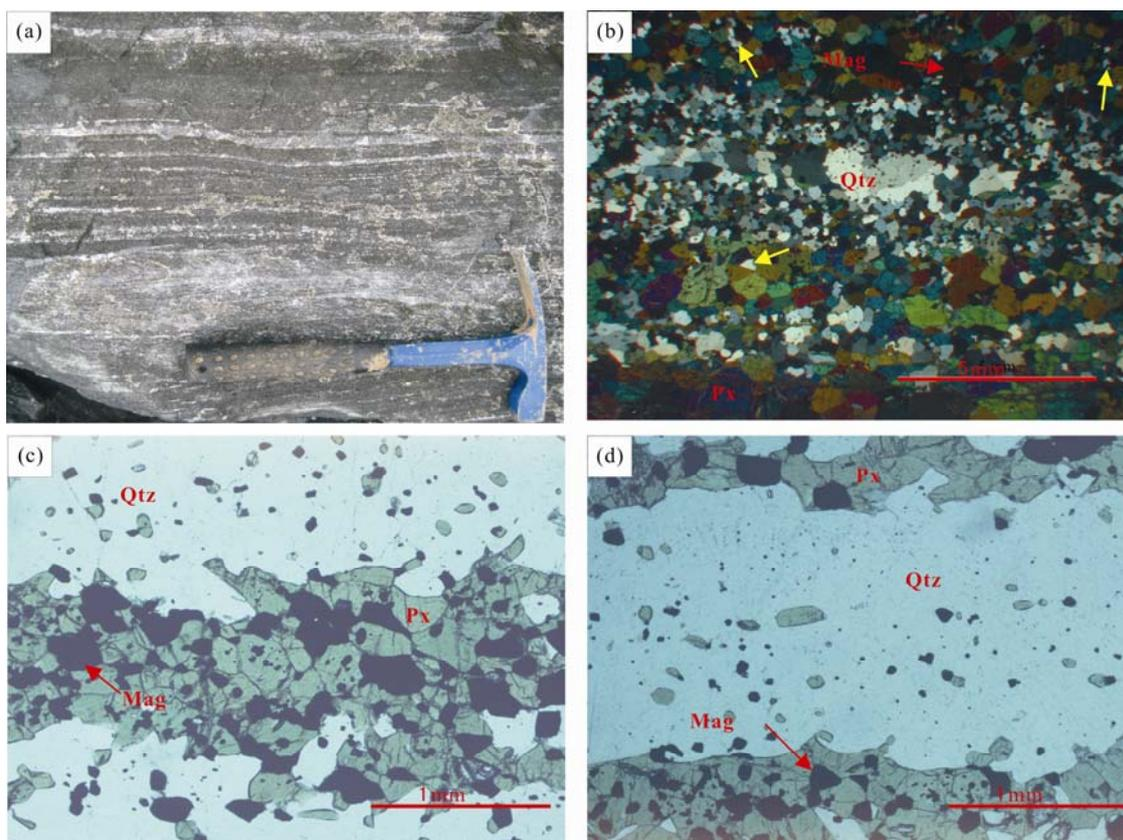
Fig. 4. Samples and microphotographs of pyroxene-magnetite BIF of the Wuyang area.
