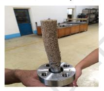
**Figure 1.** 1.5 inch steel pipe and sand pack with intelligent gel.
