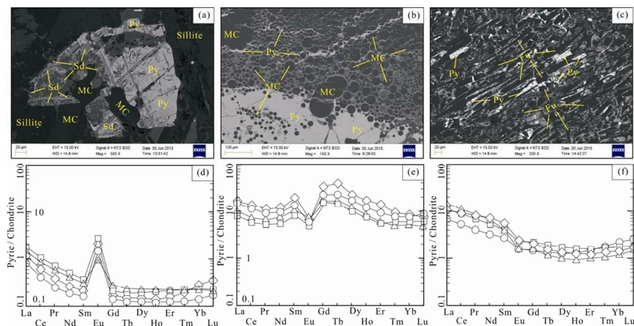
Fig. 1. Pyrite SEM images and chondrite-normalized REE diagrams of the Yangliu coal mine, northern China.
