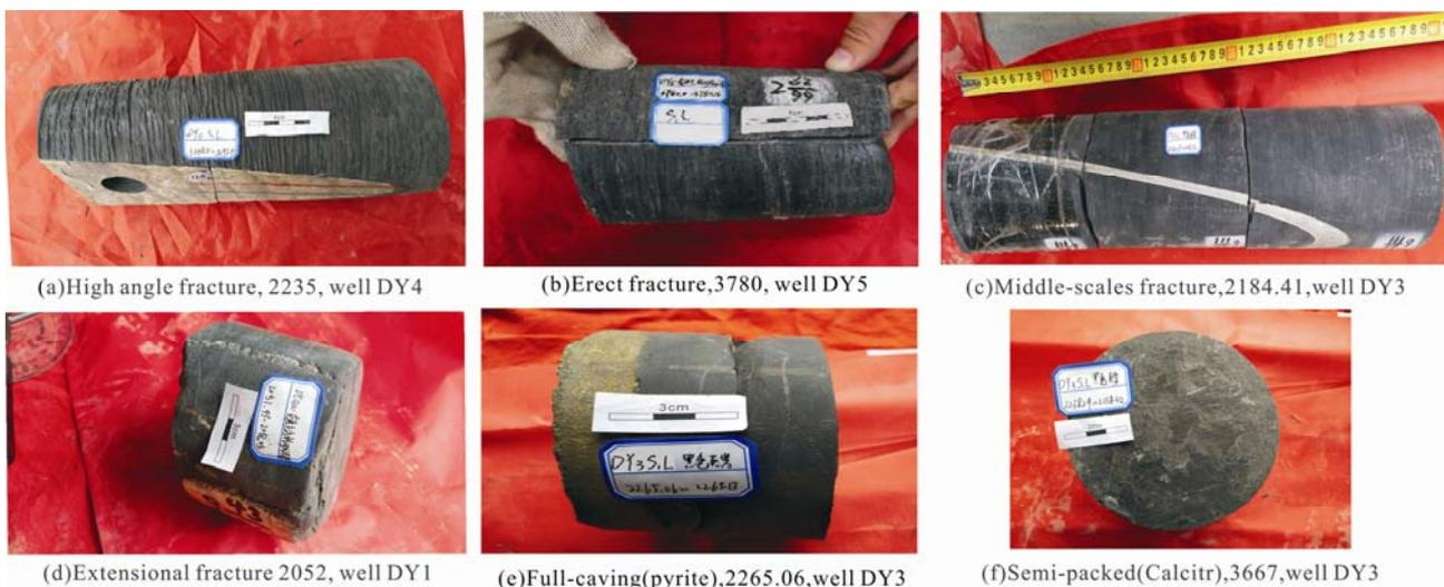
Fig. 3. Characteristics of core fractures in the Dingshan area.
