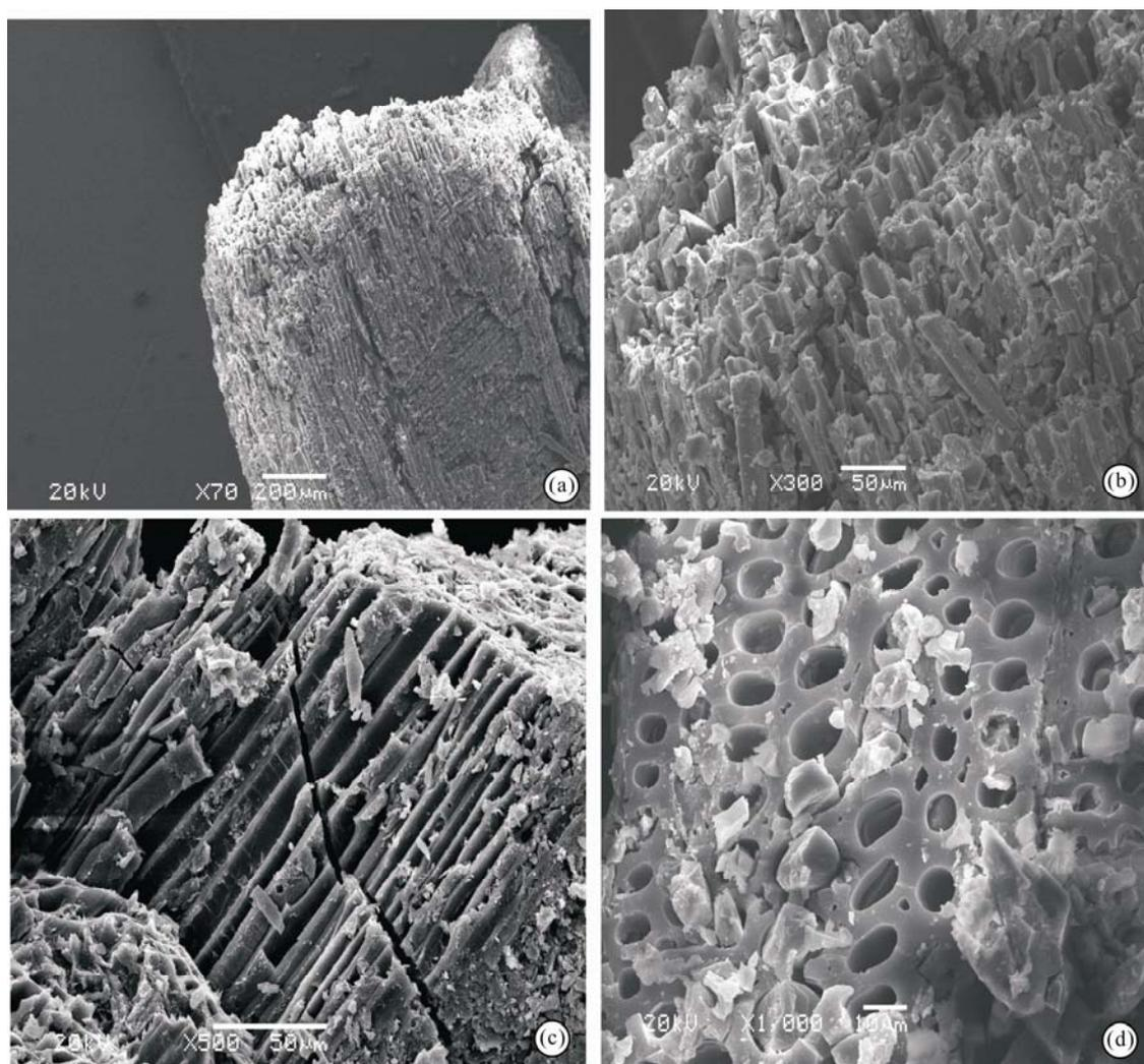
Fig. 6. SEMs of wood charcoal. (a), charcoal particle; (b, c, and d), Charred conifer wood charcoal. (b and c), tangential longitudinal section. (d), detail of tracheids showing homogenized and thick cell walls.
