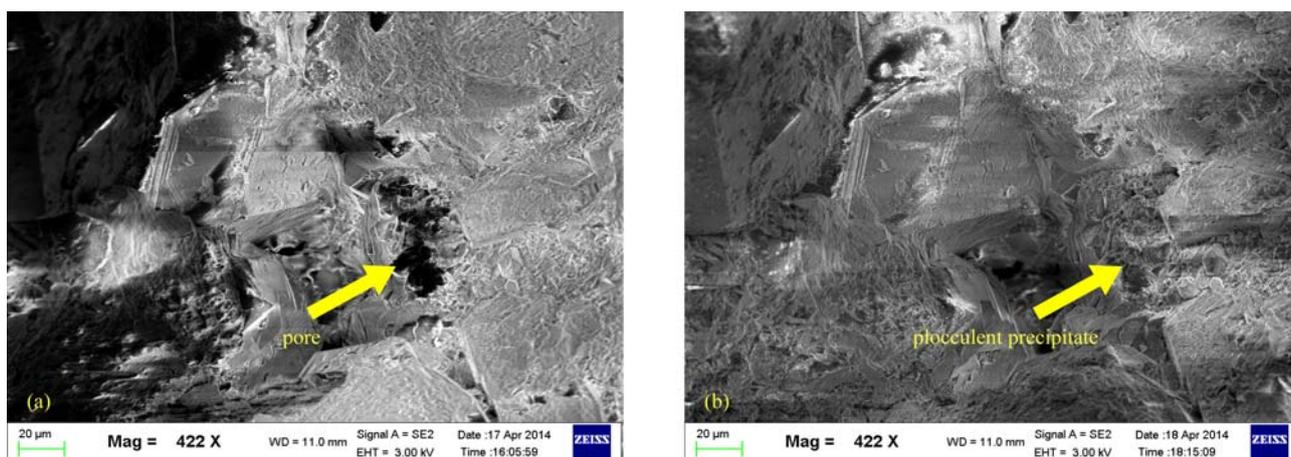
Fig. 5. Microscopic change of pores in the Kepingtage Formation before and after acid sensitivity simulation testing (26 hours immersion in 15% hydrochloric acid). (a), microscopic characteristics of initial pore before the testing (Tazhong471D, 5018.00m,  $S_1k_u^3$ ); (b), microscopic characteristics of pore after the testing (Tazhong471D, 5018.00m,  $S_1k_u^3$ ).
