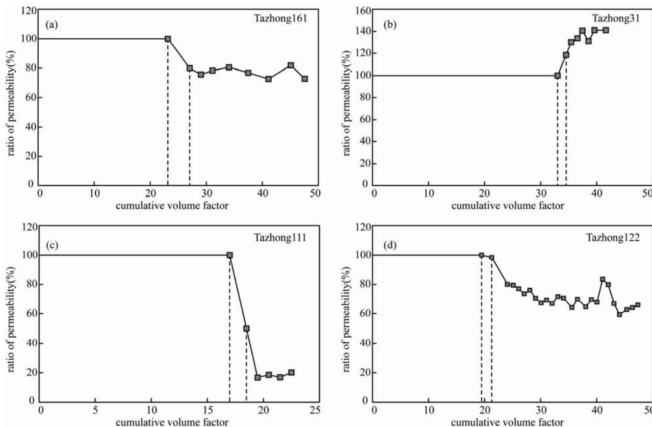
Fig. 6. Curves of acidic sensitivity of different samples in the Silurian Kepingtage Formation in Tazhong area.
