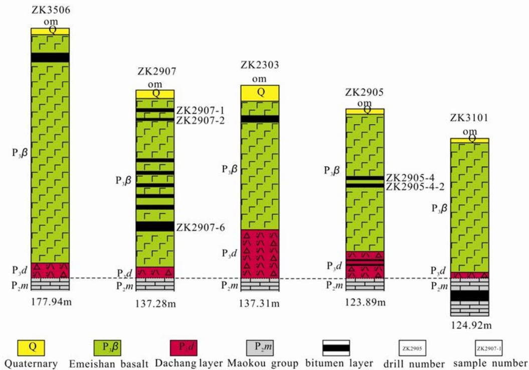
Fig. 2. The sketch map of bitumen layers in five drill holes in the Qinglong antimony deposit.
