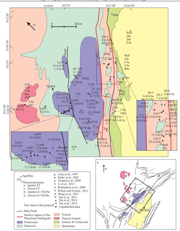
Fig. 1. (a), Geological map and low-temperature thermochronology data at the central segment of the Longmenshan thrust belt; (b), Sketch map of regional geology around Longmenshan thrust belt.
