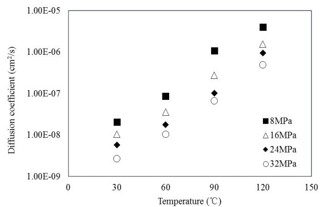
Fig. 2. Plot of methane diffusion coefficient vs. temperature for the tight sandstone in Sulige gasfield, Ordos Basin.
