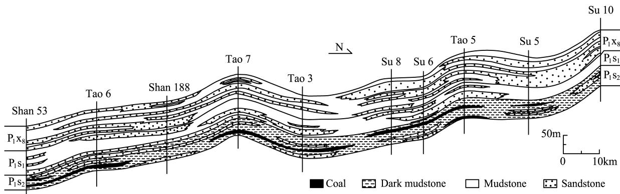
Fig. 4. Types of source-reservoir-cap rock assemblage in Sulige gasfield, Ordos Basin.
