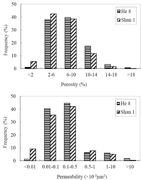
Fig. 3. Frequency of porosity and permeability of the tight sandstone in Sulige gasfield, Ordos Basin.
