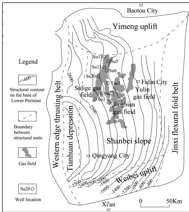
Fig.1. Structural contour map for the base of Lower Permian Shanxi Formation in the Ordos Basin and the location of Sulige gasfield (modified from Zhang et al., 2006).
