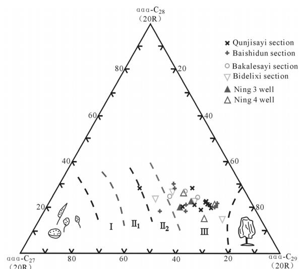
Fig. 3. Triangular diagram of organic matter type using the relative composition of sterane of Tiemulike Formation.
