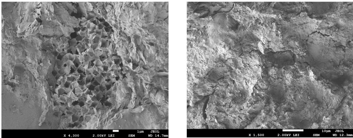
Fig. 4. A, Thermal evolution of organic matter formed honeycomb porous; B, Micro-fracture developed in black mudstone.
