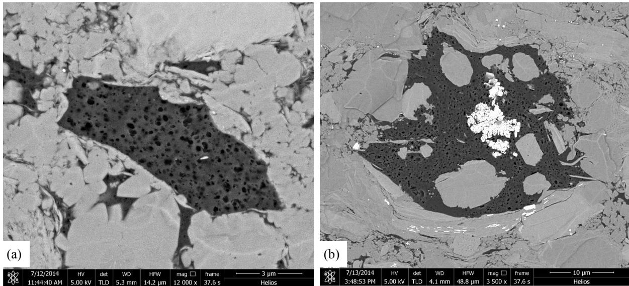
Fig. 1 Organic pore of Longmaxi shale in Chongqing Southeast (a) YC4 well 743.3m core SEM; (b) YC4 well 752.2m core SEM
