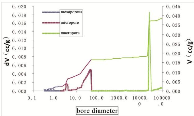
Fig. 2 Microscopic pore distribution of the full aperture in shale concluded that brittle minerals such as quartz mainly control the macro pores (> 50 nm) development, and TOC content of the shale control the organic pore development.
