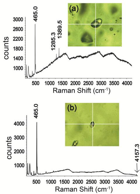
Fig. 2 Raman Spectrum of AC and AV-2 inclusions
