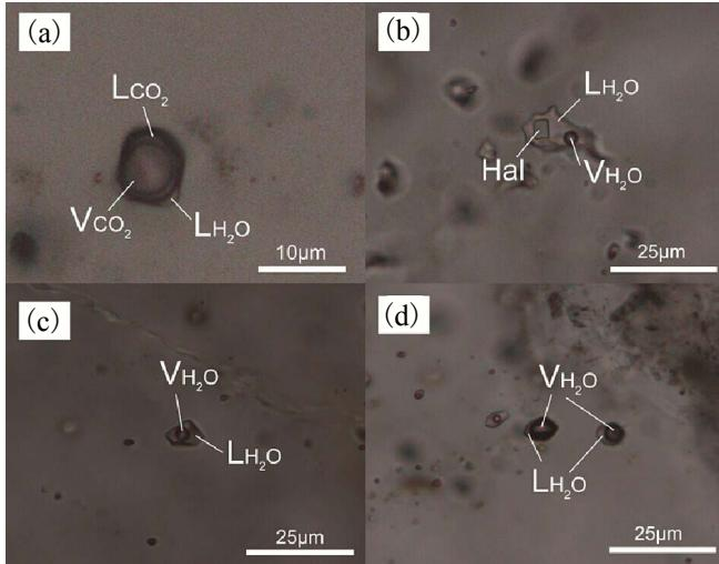
Fig. 1 Micrographs of fluid inclusions in quartz
