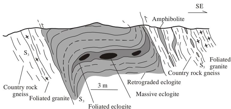
Fig. 5. Schematic cross section of the outcrop showing  $D_3$  reverse sense-of-shear indicators, such as the deflection of  $S_3$  foliation towards shear planes between retrograded eclogite and country rock gneiss, drag folds and asymmetric amphibolite boudins.
