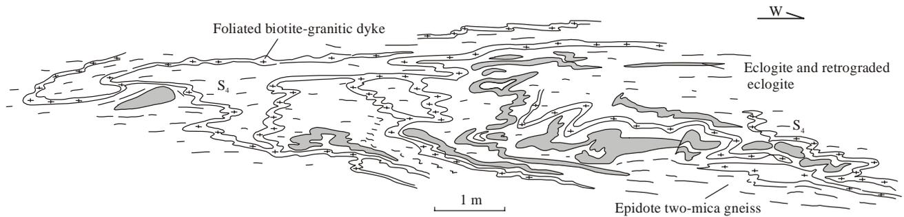
Fig. 6. Schematic E-W cross-section from the core of the Weihai structural dome, showing deformation features of foliated biotite-granitic dykes and discontinuous eclogite or retrograded eclogite layers of 10–15 cm thick in the epidote two-mica gneiss.
