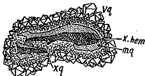
Fig. 4. Specularite (x hem) enclosed in successive layers of massive and crystalline quartz (mq & xq) forming a core on which are implanted perfect, vuggy quartz crystals (vq). Leishan, natural size.
